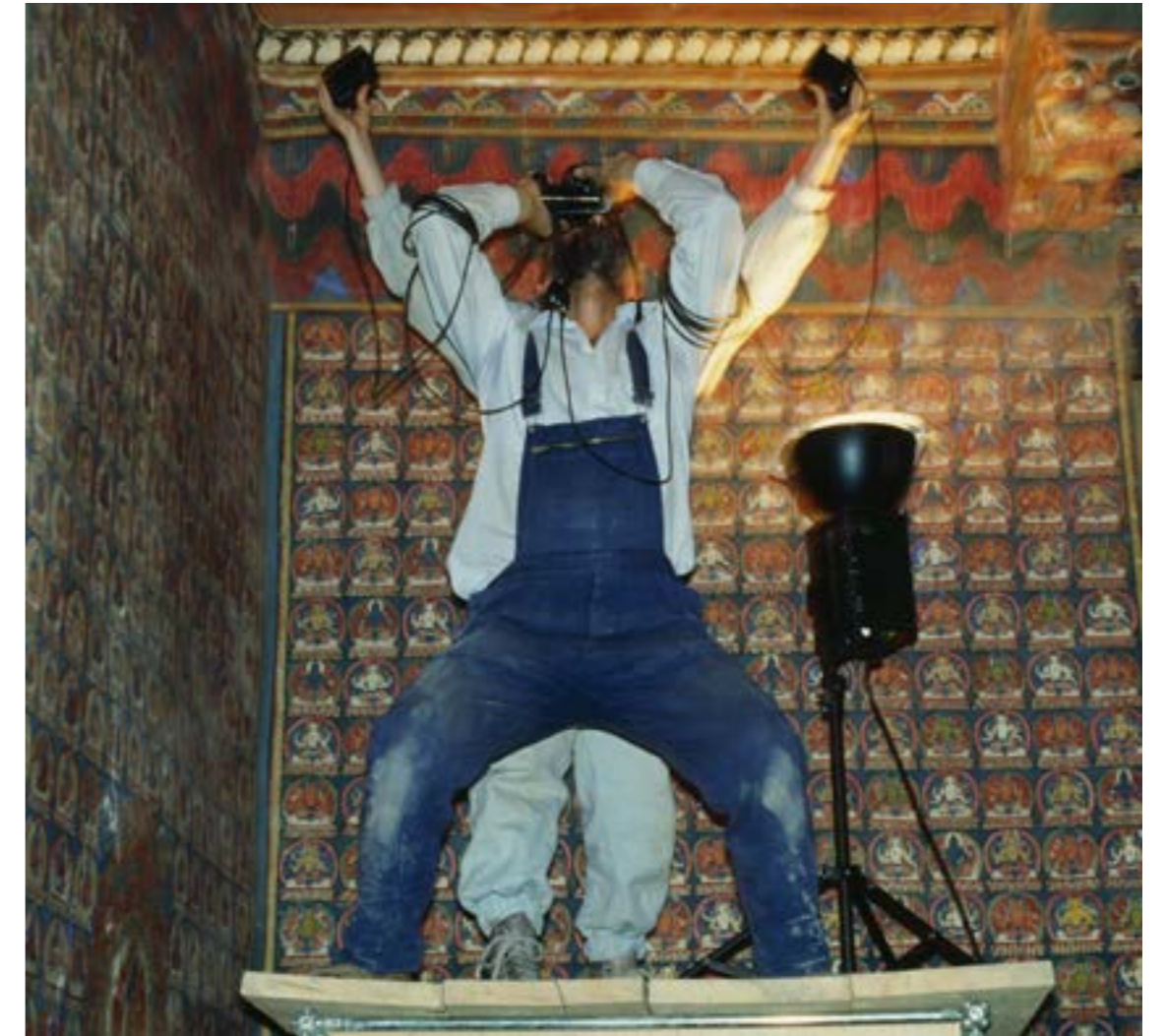
5 Jaroslav Poncar documenting a detail of a ceiling panel in the Sumtsek. Most of the documentation has been done by a simple setup of a 35mm camera with two handheld portable flash units attached to it by cables.
